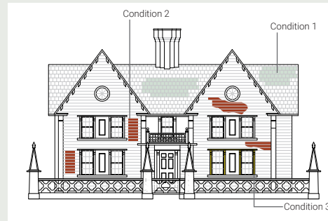
Example of an elevation drawing with annotated conditions.
