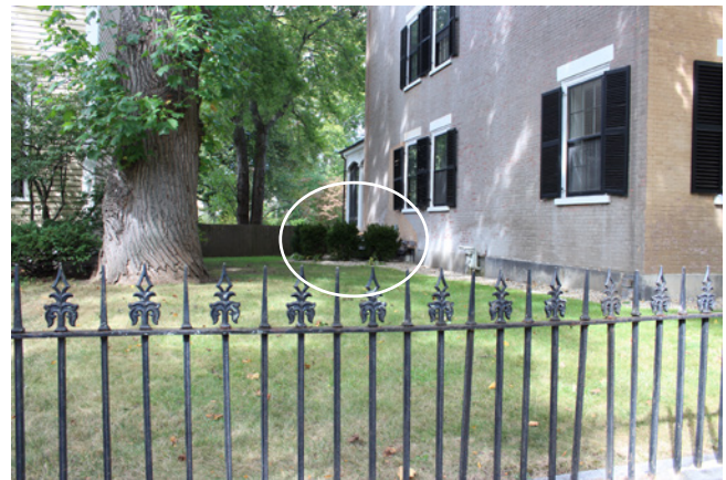
Screening equipment with landscaping and placing units far back from the street helps preserve the historic character of the building and streetscape. The location of a concealed condenser unit is circled in this example.
