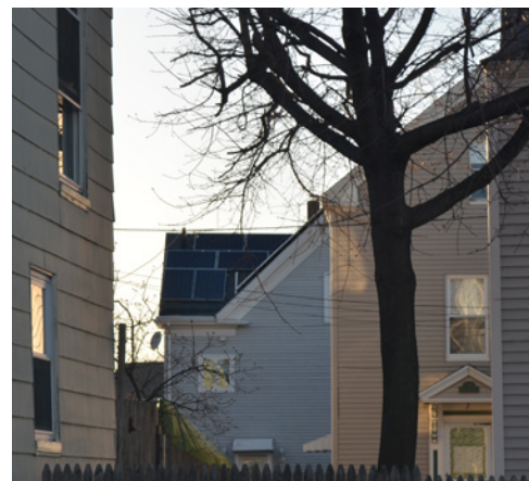
Solar panels on rear roof slopes minimize visibility from the main street. It may be unavoidable that rear panels are visible between buildings on other streets, but the immediate visual impact is reduced.
