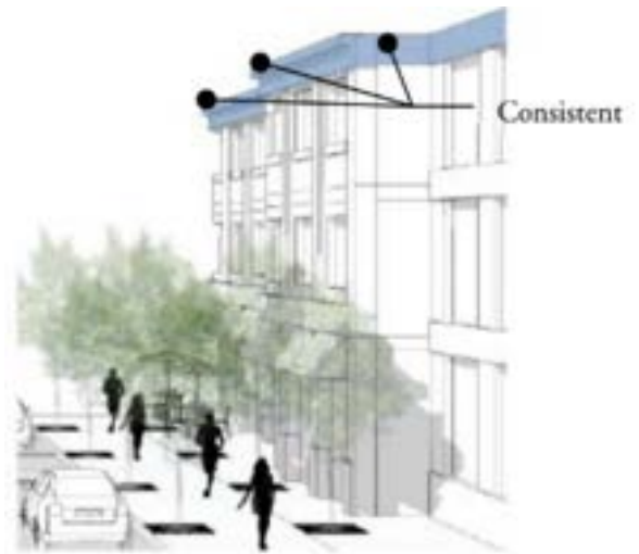
Figure 3.13 Roof Parapet and Cornice Lines
